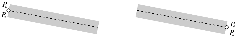
Figure 5.8: Two vertices are needed to render a stroke in the line-based drawing scheme (shown separately here). The object-space vertex position P_o is different for each vertex, while the normal N_o , and the priorities p_p and p_l are replicated (not shown). In contrast to the quad-based scheme (see Figure 5.9) the screen-space position P_s is just the projected object-space position P_o .
