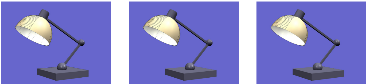
Figure 4.2: Three methods for polygon edging: edging-plane method (left, showing stitching and exposed rear edges), glPolygonOffset method (middle, no stitching but still exposed rear edges), and polygon buffer method (right, no artifacts) [Wang et al., 1999].
