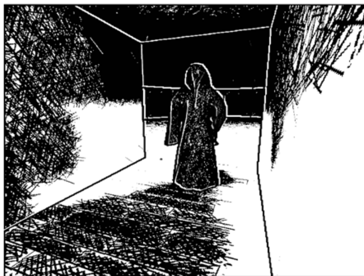
Figure 8.9: Example of a scene rendered with contrasting double contours. Note how edges are visible in both dark and light regions.
