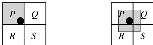
Figure 8.4: Texture sampling modes: Point-sampling chooses the nearest texel, so the color of texel P is returned (left), while bi-linear texture filtering returns the weighted average of four texels, in this example roughly \frac{4}{9}P + \frac{2}{9}Q + \frac{2}{9}R + \frac{1}{9}S (right). The exact texture coordinate is indicated as black dot, the sampling area is shown as gray square.
